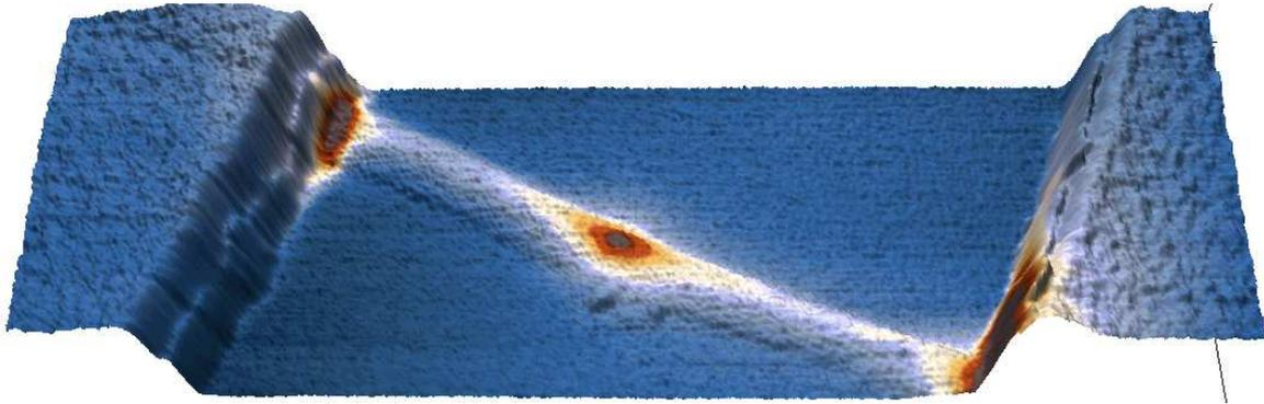
**Figure 2: Hot spots in self-heated single vanadium oxide nanowire as measured using SThM.**
