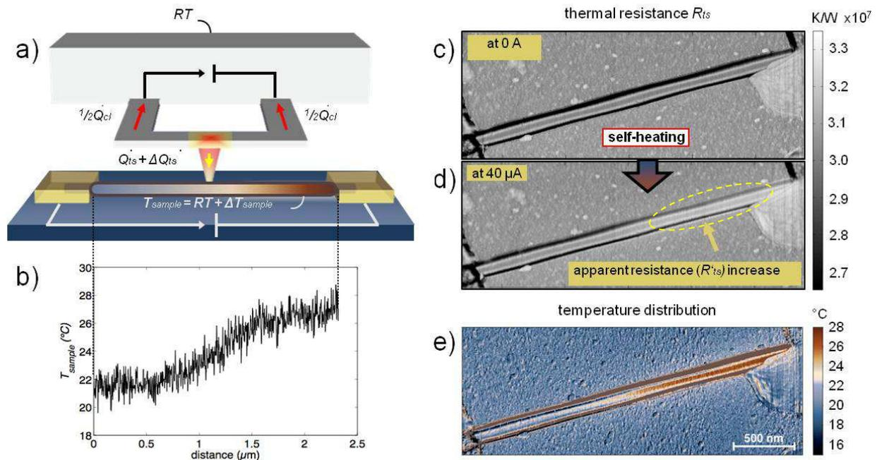
**Figure 1: Scanning thermal microscopy for thermometry of nanoscale temperature distribution.**
