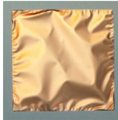
Si low stress membrane (VTT, Finland)
